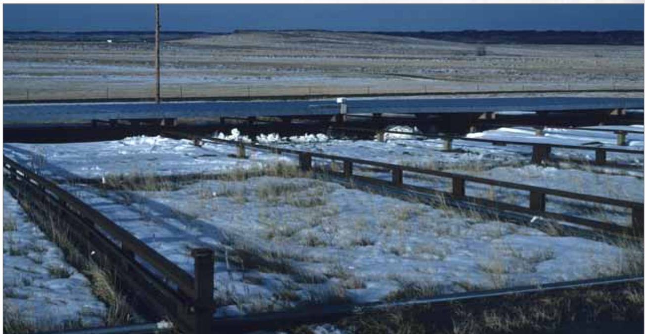
These erosion plots were used to estimate sediment production from water erosion events on mixed grass rangeland in eastern Montana.
